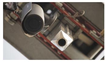
Double-wall sampling probe and camera
